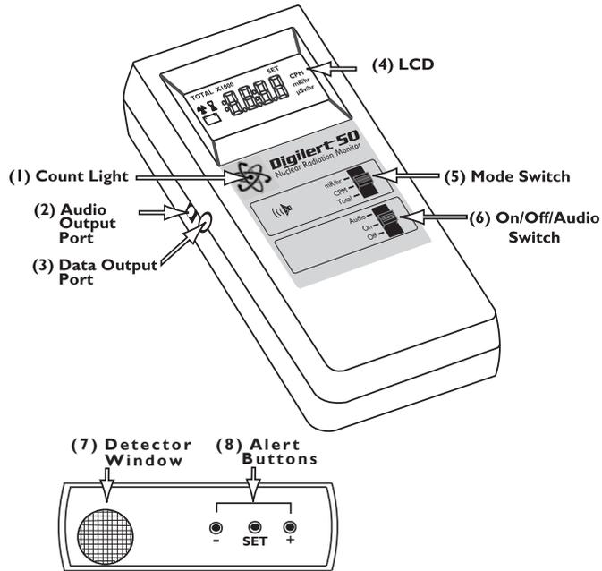
The Digilert 50 counts ionizing events and displays the results on the liquid crystal display (**LCD**) (4). You control which unit of measurement is shown by using the mode switch.
