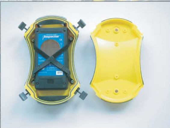
Install Inspector, centering over screen opening. Reattach the straps to hold the instrument in place
