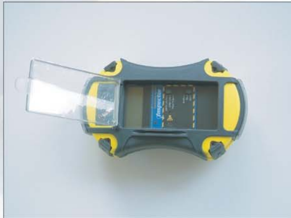
Lift hard shell window to access the Inspector controls.
