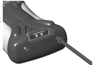
**Note:** Be sure to reattach the CF-Cap when you are finished. Recon is NOT sealed when the cap is off. Water damage caused by improper installation of the cap is not covered by warranty.
