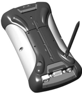
Firmly slide the PowerBoot onto the main unit as shown. Pressure should be applied downward and forward as the PowerBoot is positioned.
