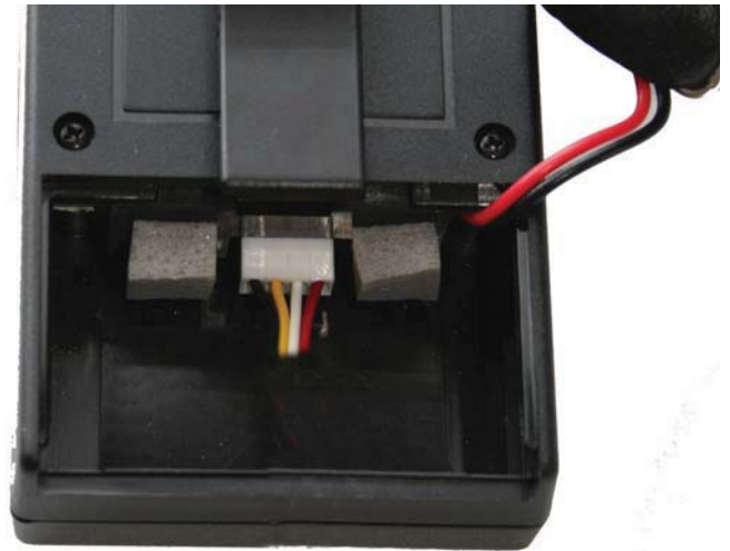
Fig 4. The Sentry - Open the battery door to connect the serial header cable that comes with the Sentry Com Software
